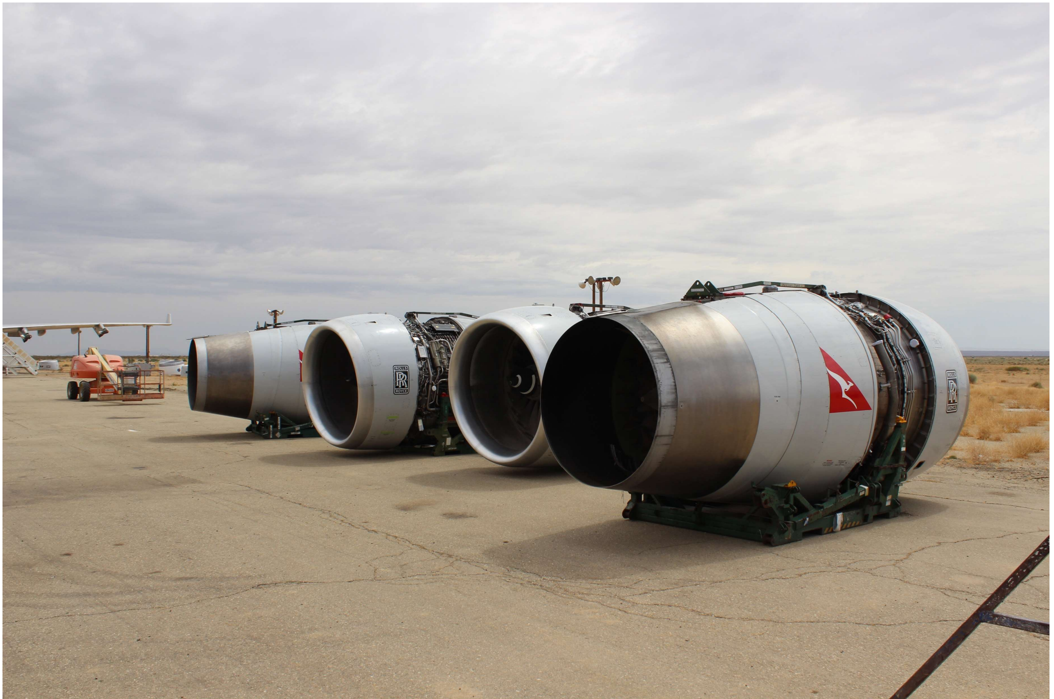
3-Aug-2017 – VH-OJM Four Rolls Engines Removed for Transport
