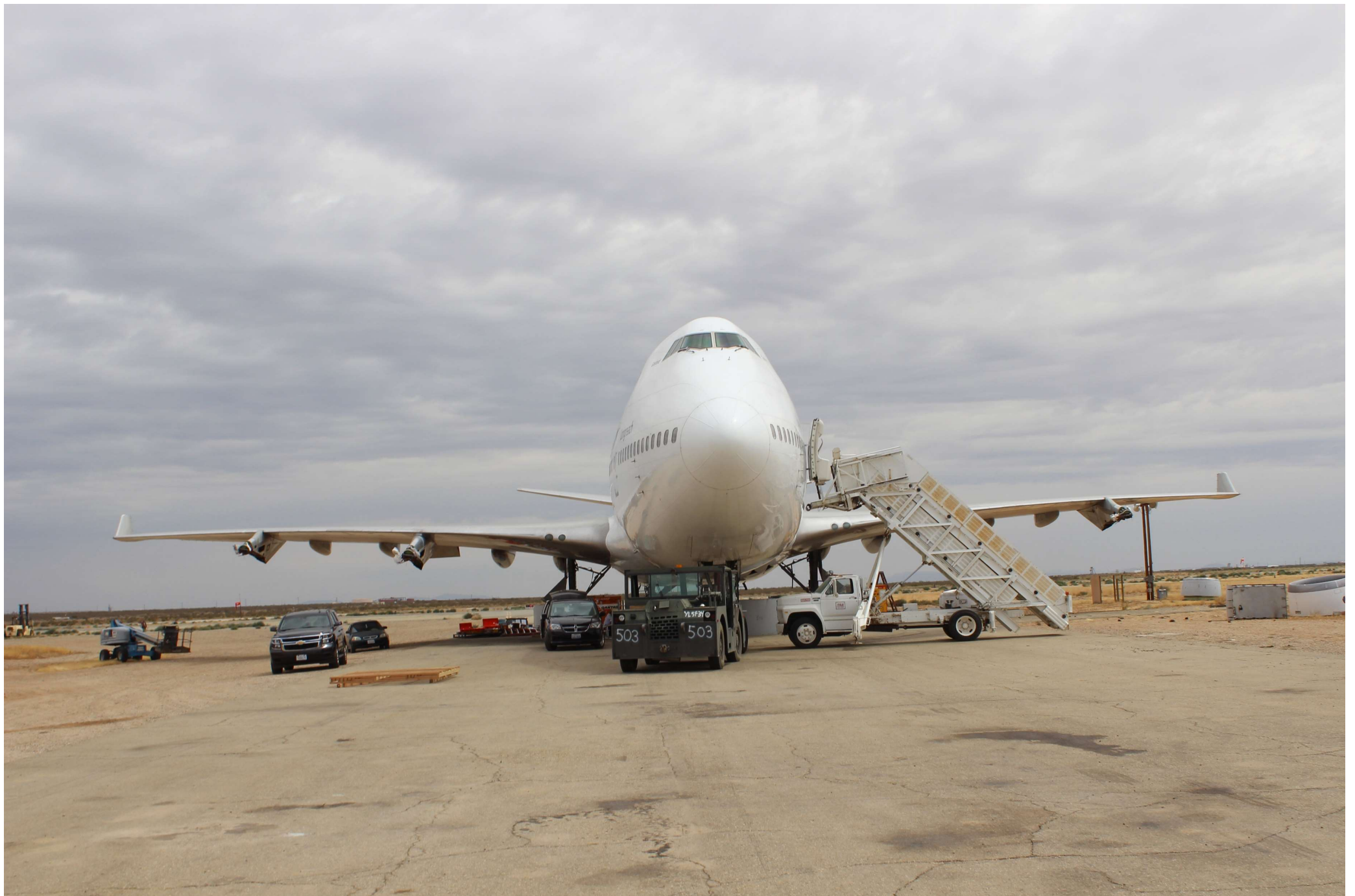
3-Aug-2017 – VH-OJM All Engines Removed
