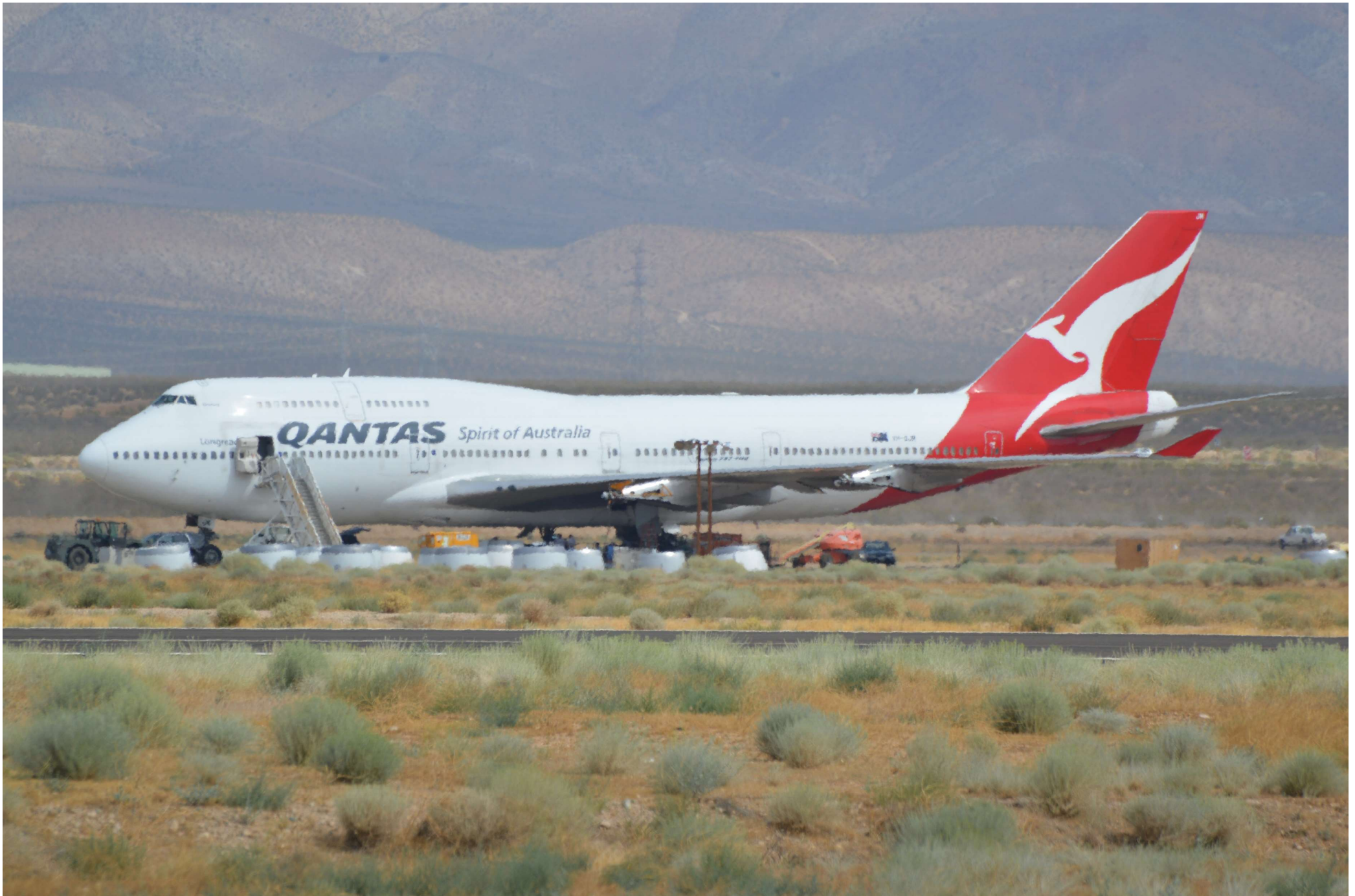
3-Aug-2017 – VH-OJM Engines Removed – Nose Cowls in Foreground
