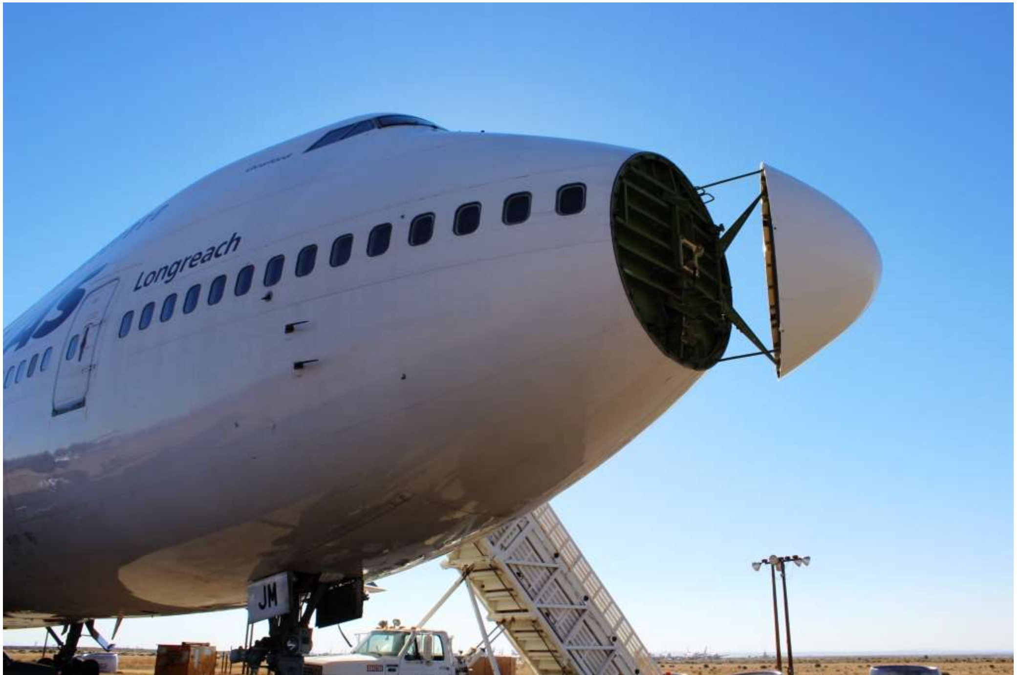
3-Aug-2017 – VH-OJM Weather Radar Removed
